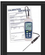
NIST Traceable Thermometer NIST traceable calibration is an assurance program that certifies that equipment is traceable to National Institute of Standards and Technology (NIST) standards and that any products offered by that manufacturer will match those NIST-maintained measurement standards. This traceability for thermometer gives greater confidence that the temperature readings are accurate.
