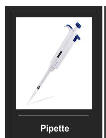
**Pipettes** may be constructed out of glass or plastic and are used to transfer a measurable amount of liquid. They are designed either to contain or to deliver a specific volume and will be stamped as such by the manufacturer.
