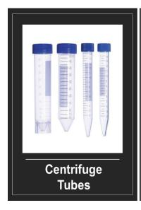
Centrifuge tubes are typically used in laboratory centrifuges, machines that spin samples in order to separate solids out of liquid chemical solutions; however, these can be used for sample collection as well.
